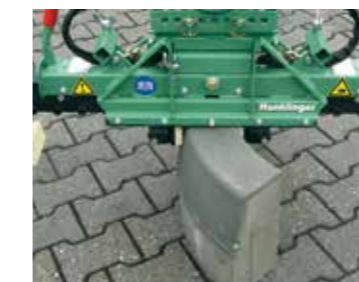
Grabbing crosswise Laying radial kerbs or picking up straight kerbs
