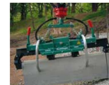
Inclination Settings Inclined laying of kerbstones
