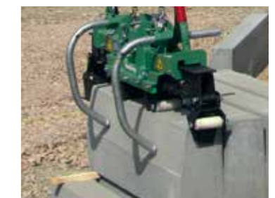
Support Bow Help for quick and easy pick up of kerbs
