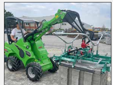
On small loaders versatile alternative to conventional laying machines
